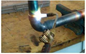
During brazing, it is imperative that the brazed joint is handled and heated properly. Additional heating and annealing of the tubes and the fitting body are not permitted.
