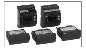
EKC 301 as DIN-rail mounting controller is designed for room temperature control via pump down or compressor start/stop. EKC 301 is controlling compressor, fan, defrost and alarm and it replaces several traditional controllers and defrost clocks due optional Real time clock module.
