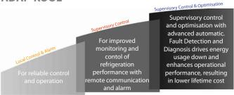
ADAP-KOOL<sup>®</sup> Refrigeration Control System is compact, flexible, easy to install and program and enables the solution to grow with the application needs. This flexible modular concept allows the constantly adaptation to the application development easy retrofitting an existing installation. ADAP-KOOL<sup>®</sup> controls offer three levels of control for different application demands with growing benefits and energy savings features according to your needs:
