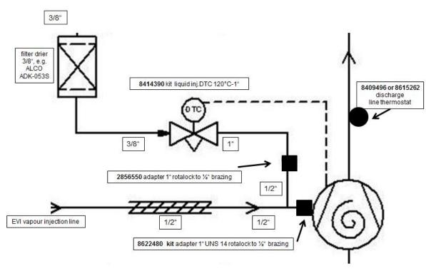
Figure 16: Installation of wet vapour injection for R407A, R407F, R448A or R449A low temp applications, example with 1/2" EVI vapour injection line
