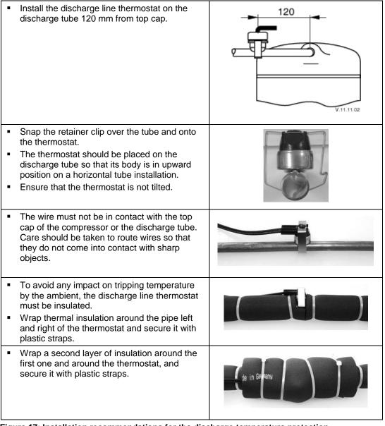
Figure 17: Installation recommendations for the discharge temperature protection
