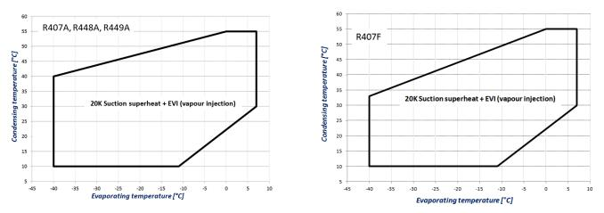
Figure 5: Operating envelopes – Vapour injection only
