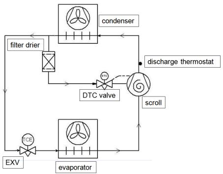
Figure 1: Liquid injection with DTC valve
