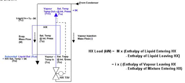
**Figure 8: Heat balance method for calculating the HX load and injection mass flow rate** C7.19.2/0813-1016/E
