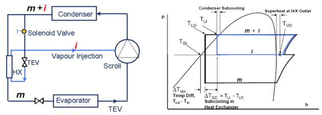
Figure 6: Circuit diagrams showing the main circuit, the mass flow rate m, the economizer circuit and the mass flow rate i
