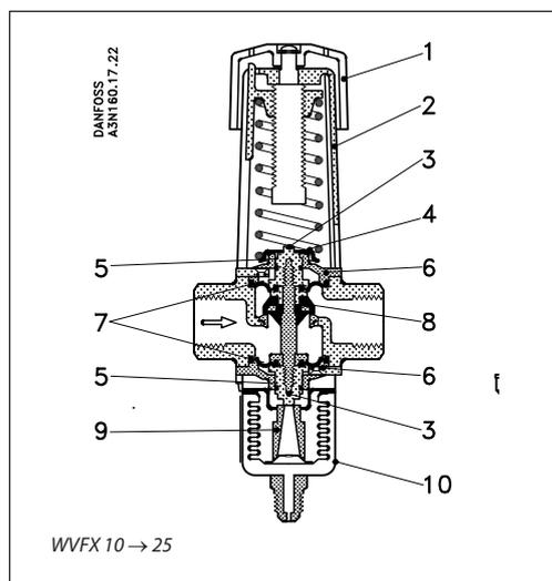
The valve plate (8) is a brass plate with a vulcanized layer of special rubber to form an elastic seal against the valve seat. The valve is externally sealed by the diaphragms (7).
