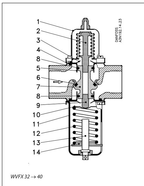
The valve cone (7) is made of brass with a T-ring (6) of artificial rubber forming a flexible seal against the valve seat.
