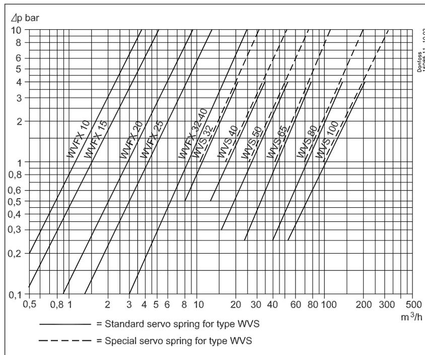
The capacity curves show the capacities of individual valves (water quantity in m<sup>3</sup>/h) depending on the pressure drop across valves.
