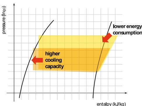
The extended operating range of the E<sup>V</sup> means the refrigeration unit can work with floating condensing pressure, and consequently at the minimum allowed for the ambient temperature. This brings significant energy savings in all refer applications.
