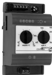
This module converts a temperature input signal to a standardised output signal of 0 to 10 or 4 to 20 mA. The input signal can either be obtained from a temperature sensor or a temperature control module. The signal converter can be used for those applications where an analogue output is required. Such as; to a motor, motor actuated valve, recorder etc.
