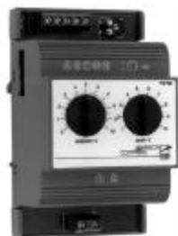
This module converts a voltage input signal to a standardised output signal of 0 to 10 Vdc or 4 to 20 mA. The input signal can either be obtained from a pressure sensor or a pressure control module. The signal converter can be used for those applications
