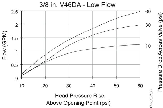
**Figure 6: 3/8 in. V46 Direct-Acting Low Flow**
