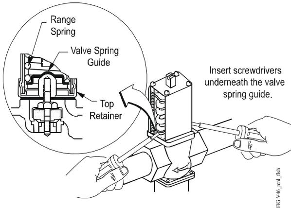
**Figure 19: Manual Flushing**
