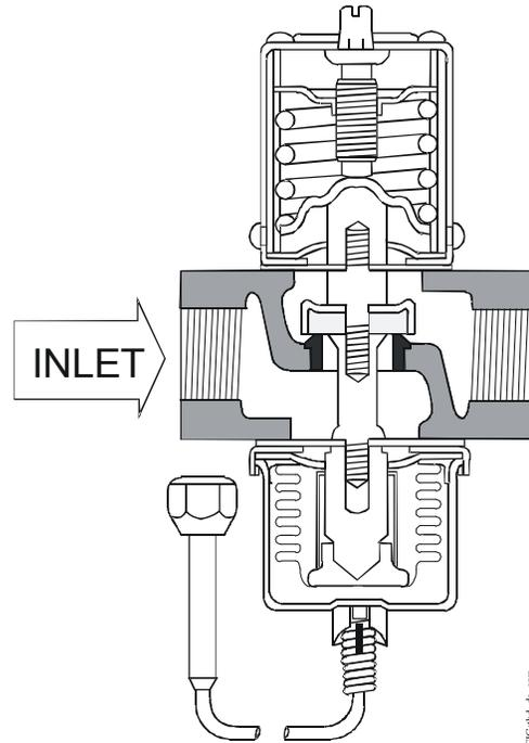
Figure 2: Threaded Type Direct-Acting Valve Cross Section
